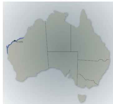
Figure 12: Region D as identified by the Building Code of Australia, which requires buildings to withstand cyclones up to a category 5 with 280 km/hr wind
