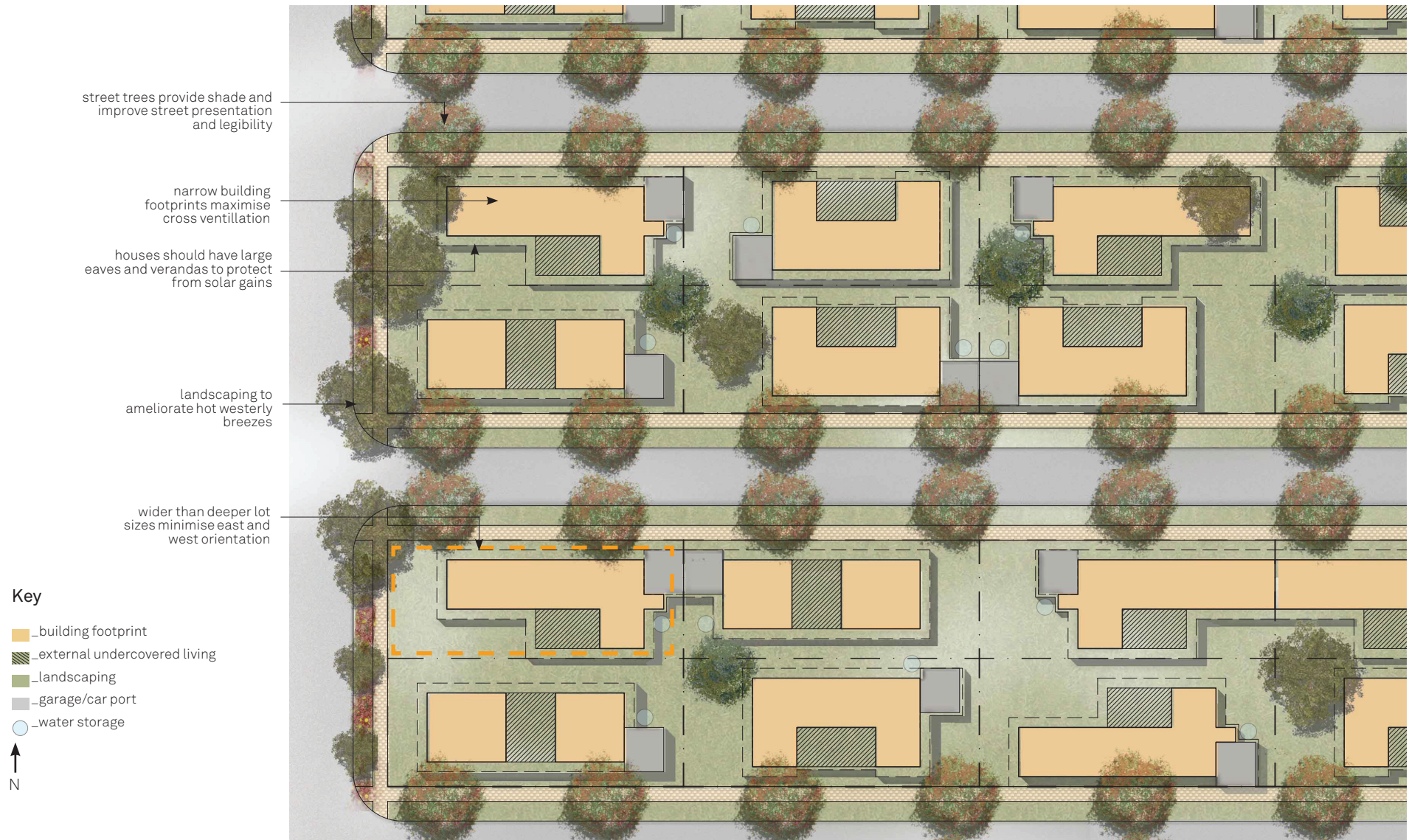
Figure 20: Lot design and orientation for Mulataga needs to facilitate passive design for houses, as shown here, as well as for denser residential development.
